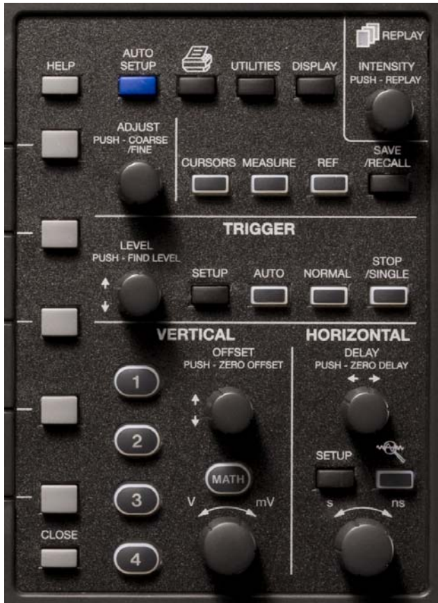
Figure 1: The front panel of a WaveJet. When something interesting appears on the screen the user can press “stop” trigger and then rotate the Replay knob (upper right) to view or measure up to 1024 recent individual waveform acquisitions.
