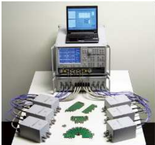
1. This 12-port VNA system makes mixed-mode and balanced differential S-parameter measurements from 40 MHz to 65 GHz.
