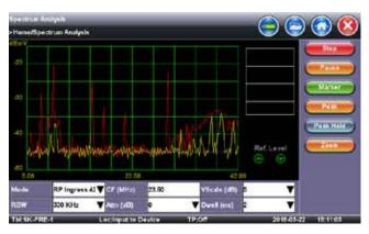
The CX350s-D3.1 is equipped with powerful spectrum analyzer features including a high dynamic range, markers, peak hold, variable resolution bandwidth (RBW) and variable dwell time (sweep speed) to help troubleshoot, identify and fix interference related problems.
