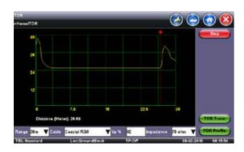
The cable under test is scanned within seconds, allowing the user to view the full run and to identify faults quickly.
