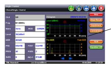
The histogram feature records level, MER, Pre-BER, Post-BER, and Error seconds on per second time bucket for up to 60 minutes. The results are shown in graphical format that allows easy correlation of measured parameters down to one-second resolution.
