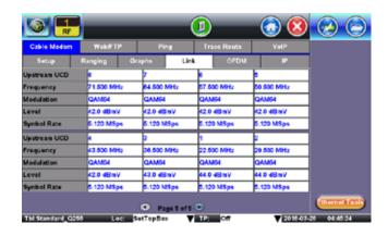
For advanced troubleshooting, Upstream Pre-Equalization Adaptive EQ parameters can be viewed by tapping on the desired UCD number.
