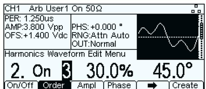
*The harmonics generator enables waveforms to be constructed using up to 16 sine harmonics*
