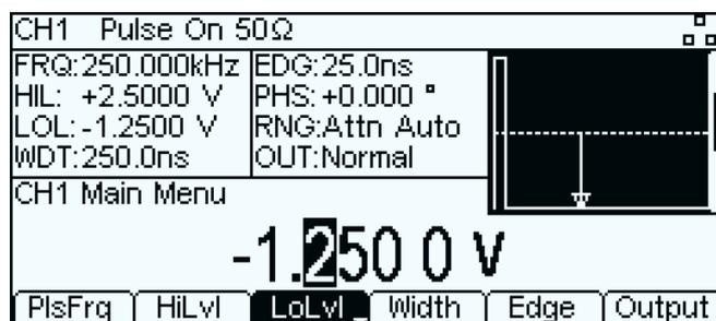
Output levels can be entered as high level and low level as an alternative to amplitude and offset
