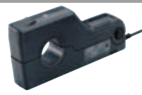
UNIVERSAL CLAMP ON CT 9279-01 (CE marked) 500A AC/DC φ40mm (1.57") POWER SUPPLY: 9555-10
