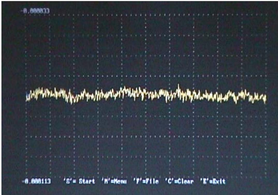
Transducer Signal. Iout = 0A. Vertical scale 150uA/div.
