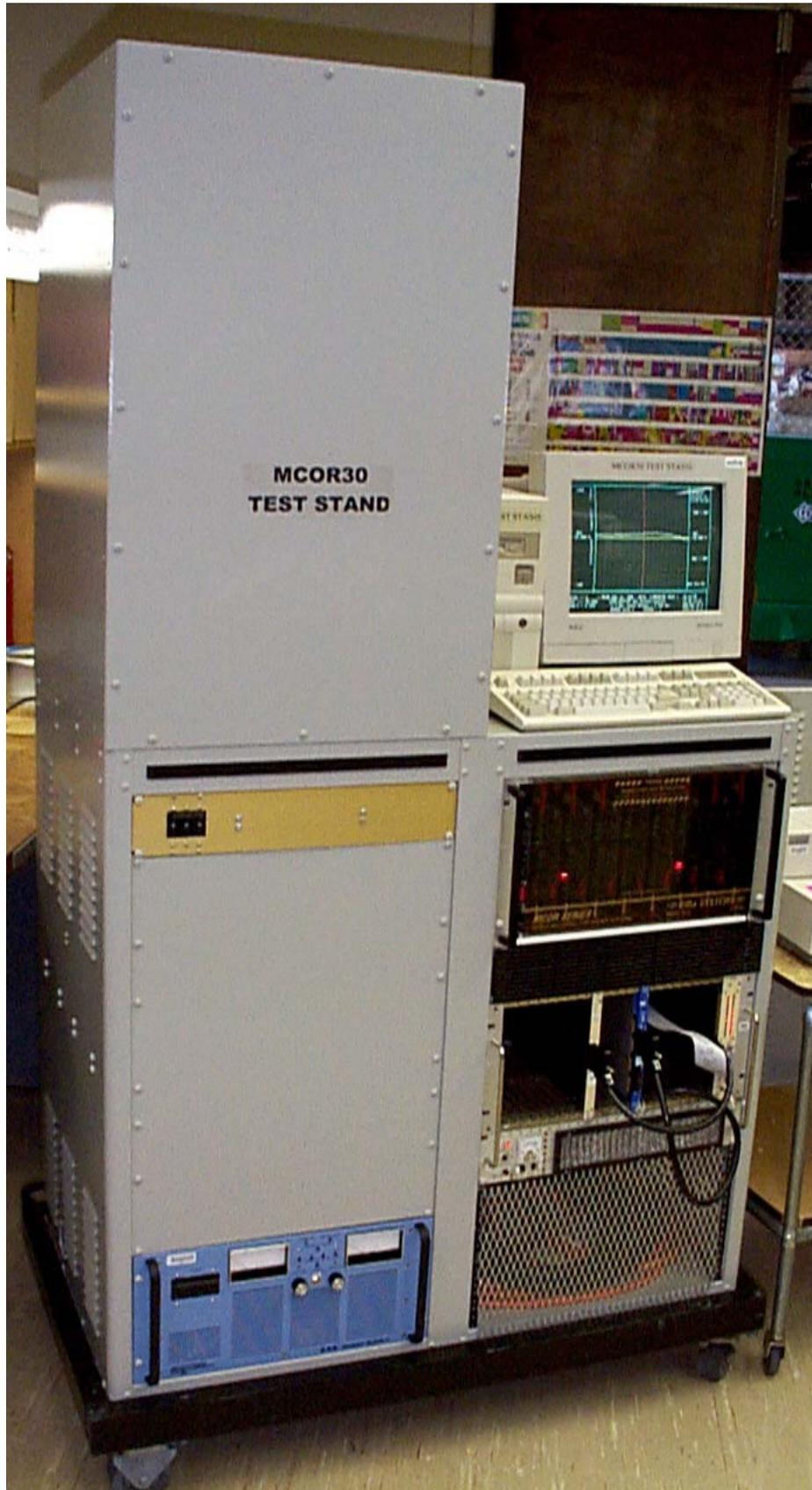
**Figure 4.0. The MCOR30 DVIG Test Stand.**
