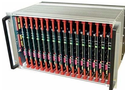
Figure 1: Shows MCOR crate load with 16 Power Modules and interface card on far left.
