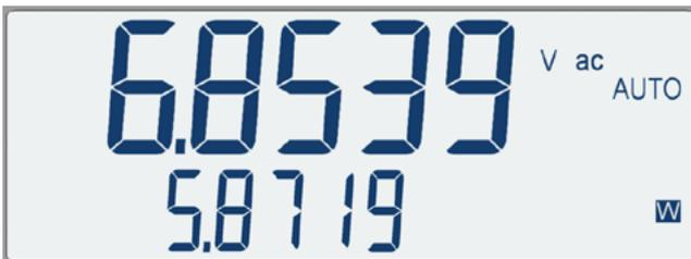
The VA function makes use of the dual measurement capability and displays the product of voltage and current.
