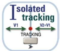
The two outputs of the CPX are completely independent and electrically isolated from each other. With V-Track selected, the two outputs remain electrically isolated, but the voltage control of the Master output sets an identical voltage on the Slave output.
