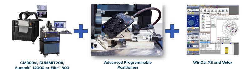
**Autonomous RF measurement assistant -** Sophisticated optical alignment algorithms combine with high-precision programmable positioners automate the probe to pad alignment of the RF and DC probes on the device under test and calibration substrate
