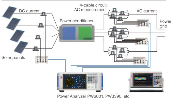
Once a current sensor has been attached to each branch cable, the CT9557 adds the sensor signals together to create a total signal. Since the device can treat multiple sensors as a single sensor, as illustrated in the figure above, the current can be measured using a single power meter.
