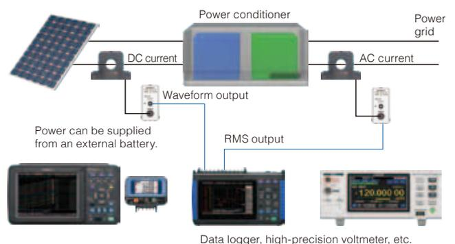
In this setup, waveform output is monitored on the DC current side, and RMS output is monitored on the AC current side of the circuit. Even a logger that lacks RMS conversion functionality can be used to measure AC current. A wireless logger can also be used. If a high-precision voltmeter is used, both the AC and DC currents can be measured with a high degree of precision.
