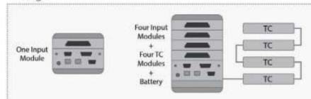
A single Echelon system can be configured as small as one input module and processor module or as large as 4 input modules, 4 thermocouple satellites, and a battery. A single Processor Module supports up to 64 channels at 100 kS/s per channel, 128 channels at 20kS/s per channel, or 16 channels at up to 1 MS/s per channel.
