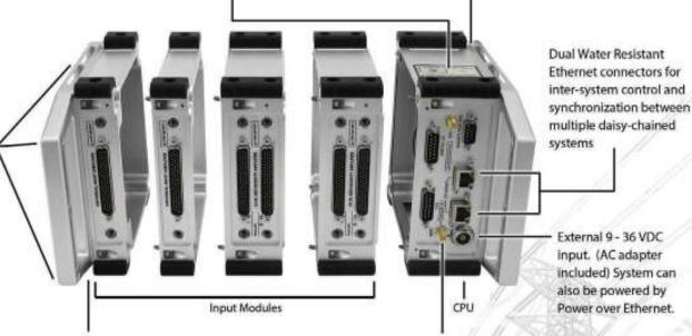
Sealed modules and gasketed interconnects support IP 67 Environmental rating Wireless 802.11 provides simple external control, monitoring and setup from most wireless devices. Optional high gain antenna supports communication up to 1000 meters
