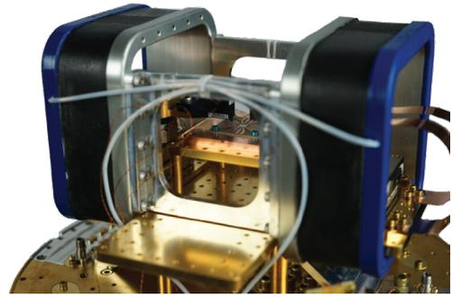
Create the right sample environment with options such as horizontal and vertical magnetic fields.
