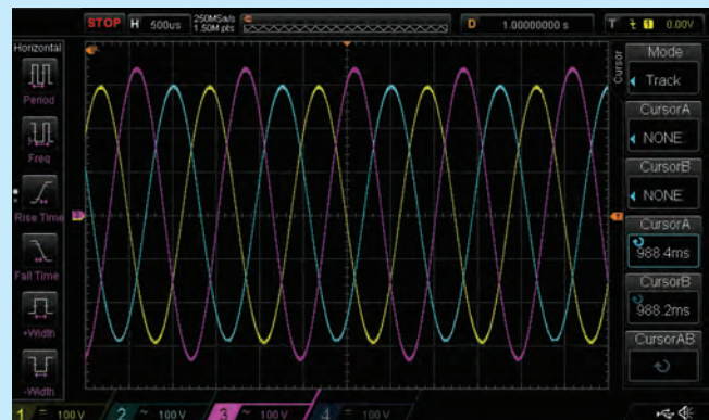
Three Phase Unbalance Voltage Test Captured
