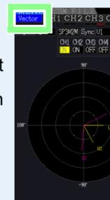
This page displays measured harmonic voltage, harmonic current, and harmonic power on channels 1 to 4 as numerical values and as vectors.
