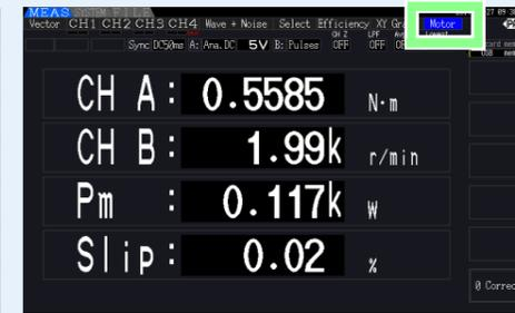
This page displays measured values for the motor analysis function.
