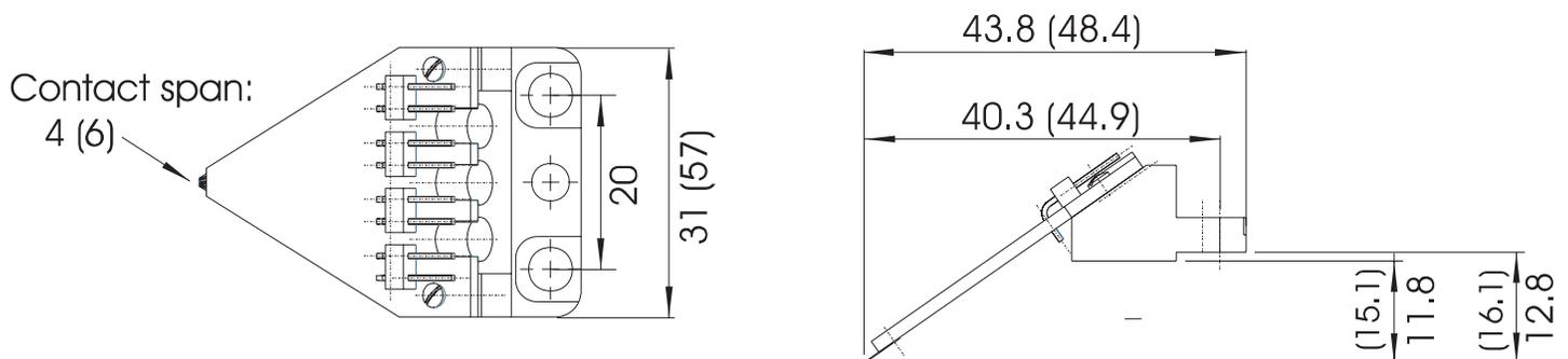
Multi |Z| Probe 3 to 7 pin with medium board size. Variational figures for Multi |Z| Probe 7 to 25 pin with large board size in brackets.
